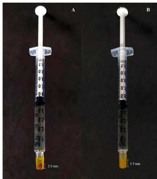
Figure 7. Physical structural model to evaluate antibacterial activity of chayotextle starch-based film functionalized with a multi-herbal formulation. A) Syringe is treated with iodine-based sealant. B) Syringe is treated with CSF-MHF.
