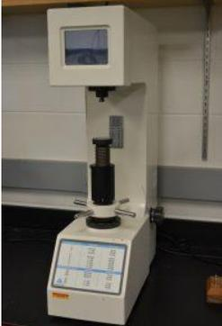
A vertical hardness testing machine with a digital display and a control panel.                 |
