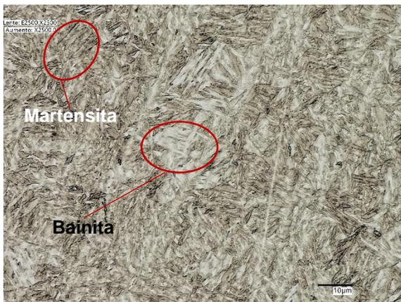
Figura 31. Acero 4140 a 2500X/Nital3%/3s/Keyence. Colonias de martensita y bainita.
