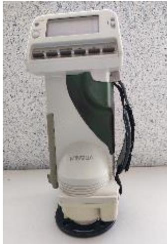
**Figura 14.** Colorímetro MINOLTA CM-2002 SPECTROPHOTOMETER.
