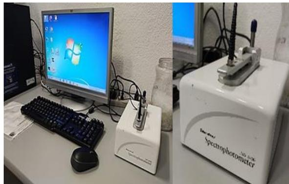
**Figura 16.** NanoDrop 1000 (NanoDrop Technologies) Spectrophotometer V3.8.
