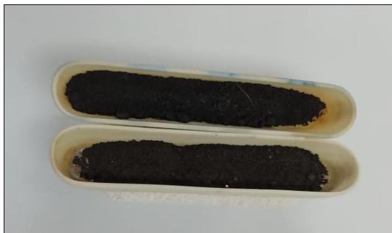
**Figura 4.1** Macrofoto de los polvos sintetizados: (a)  $\text{La}_{0.7}\text{Ca}_{0.2}\text{Sr}_{0.1}\text{MnO}_3$  y (b)  $\text{La}_{0.7}\text{Sr}_{0.3}\text{Mn}_{0.8}\text{Cr}_{0.2}\text{O}_3$ .
