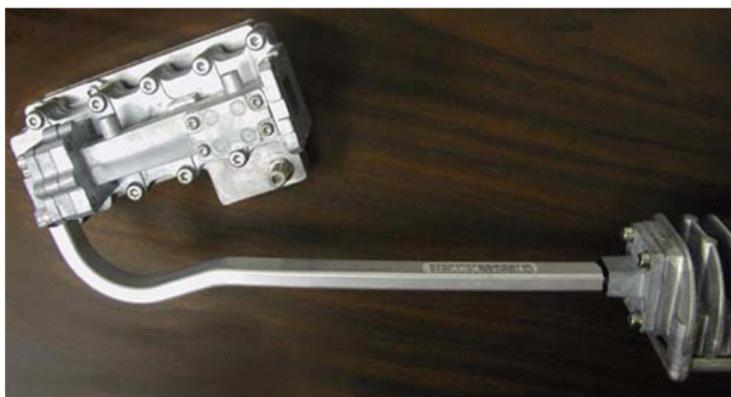
Figura 2.7: LNB (Low Noise Block)
