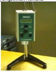
VISCOSÍMETRO Modelo DV-E, Brookfield Ingineering Laboratories, Inc. EU
