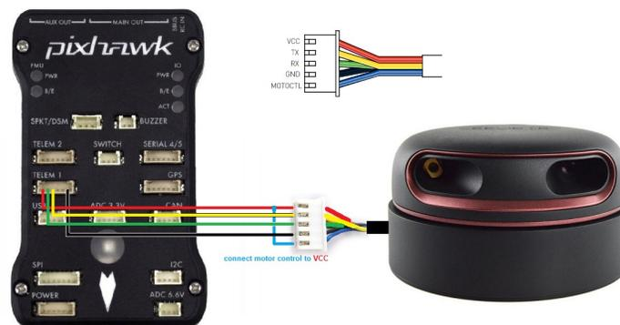
Figura B.2: RPlidar PIX-HAWK® pinout [22].
