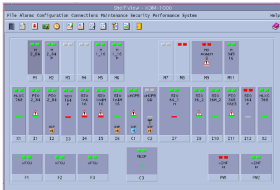
Figure 3-26: Typical XDM-1000 shelf view window
