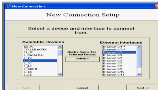
Figura 6.235 Interfaz ethernet 0/3 del switch S_2C
