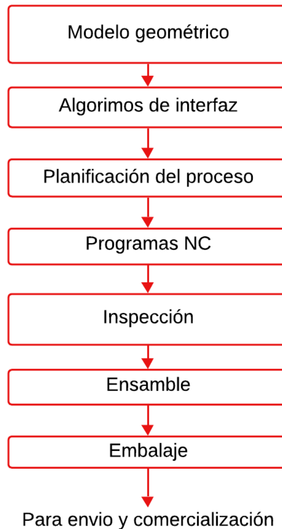
Figura 7. The CAM process. Fuente CAD/CAM: Concepts and Applications.
