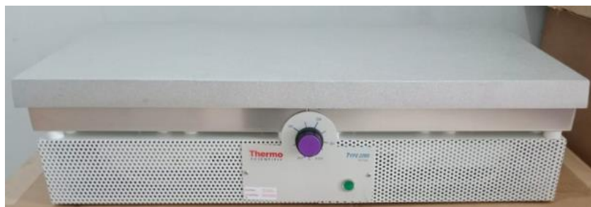
Figura 18. Platina térmica Thermo Scientific Thermolyne HPA2240MQ ( Thermo Scientific Thermolyne HPA2240MQ Aluminum Hot Plate, 24" X 12", Di ANDALAN LABSTORE | Tokopedia,s.f )
